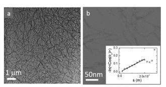
Fig. 2 (a) Cryo-TEM image of the hexamer  $\mathbf{1}_6$  after one month, showing the hydrogel network structure. Concentration of 1 was 3.8 mM. (b) Negative staining electron microscopy image of the same fibers after diluting 100 times. The image shows individual fibers. Inset:  $-\ln\langle\cos(\theta_{ij})\rangle$  obtained by fitting splines to the fiber contours in a dilute fiber suspension as a function of arc length. The persistence length is obtained from the slope of a linear fit
