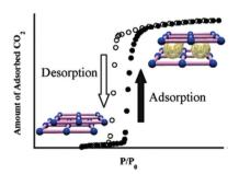
Fig. 17 Schematic representation of clathrate formation during CO<sub>2</sub> adsorption. Reproduced with permission from ref. 57, Copyright (2006) American Chemical Society.
