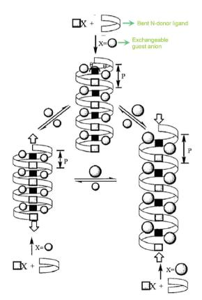
Fig. 2 Helical pitch tuning by anion exchange in a cationic solid. Reproduced with permission from ref. 30, Copyright (2000) American Chemical Society.
