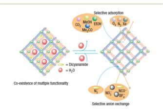
Fig. 3 Schematic illustration of mutual sliding of nets induced by anion exchange in a cationic MOF. Reprinted with permission from ref. 32, Copyright (2007) Macmillan Publishers Ltd.
