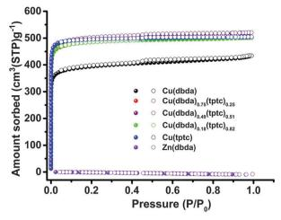
Fig. 3 N<sub>2</sub> gas sorption of  $Cu(dbda)_x(tptc)_{1-x}$  (x = 1, 0.75, 0.49, 0.18, 0). Adsorption and desorption branches are shown with filled and empty symbols, respectively.
