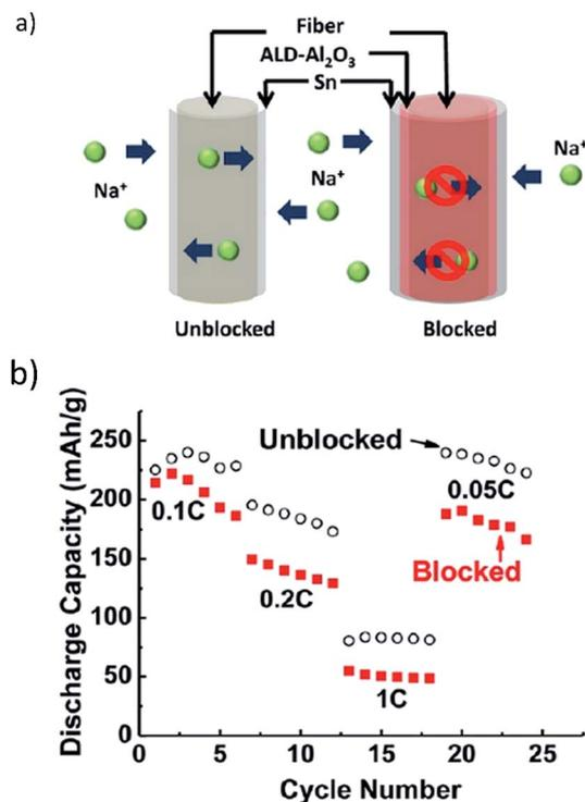
Fig. 13 (a) Na ions transport along and diffuse through the mesoporous wood fiber structure. Internal transport pathways are blocked by the conformal Al<sub>2</sub>O<sub>3</sub> coating, and (b) the rate performance of the Sn anode deposited on the carbon-coated mesoporous wood fibers. Reproduced with permission<sup>137</sup> © 2013, ACS Publications.
