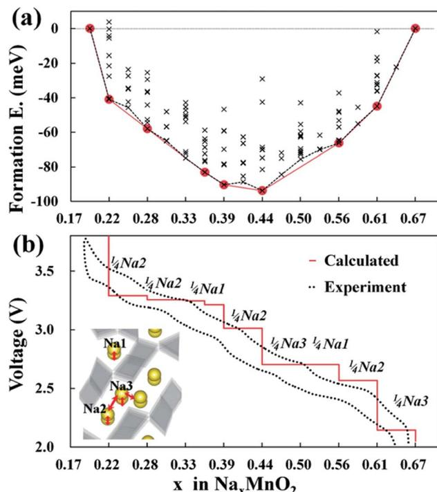
Fig. 6 (a) Formation energies of seven stable intermediate phases during  $\text{Na}_x\text{MnO}_2$  cycling calculated from 156 different sodium configurations, and (b) experimental and calculated voltage profiles for  $\text{Na}_x\text{MnO}_2$  with respect to the minimum energy path of formation energies. Reproduced with permission<sup>55</sup> © 2012, ACS Publications.
