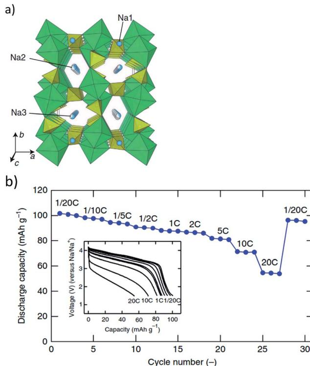
Fig. 8 (a)  $\text{Na}_2\text{Fe}_2(\text{SO}_4)_3$  structure projected along the *c* axis, and (b) capacity retention upon cycling up to 30 cycles under various rate of  $\text{C}/20$  (2 Na in 20 h) to  $20 \text{ C}$ . Reproduced with permission<sup>80</sup> © 2014, Nature Publishing Group.
