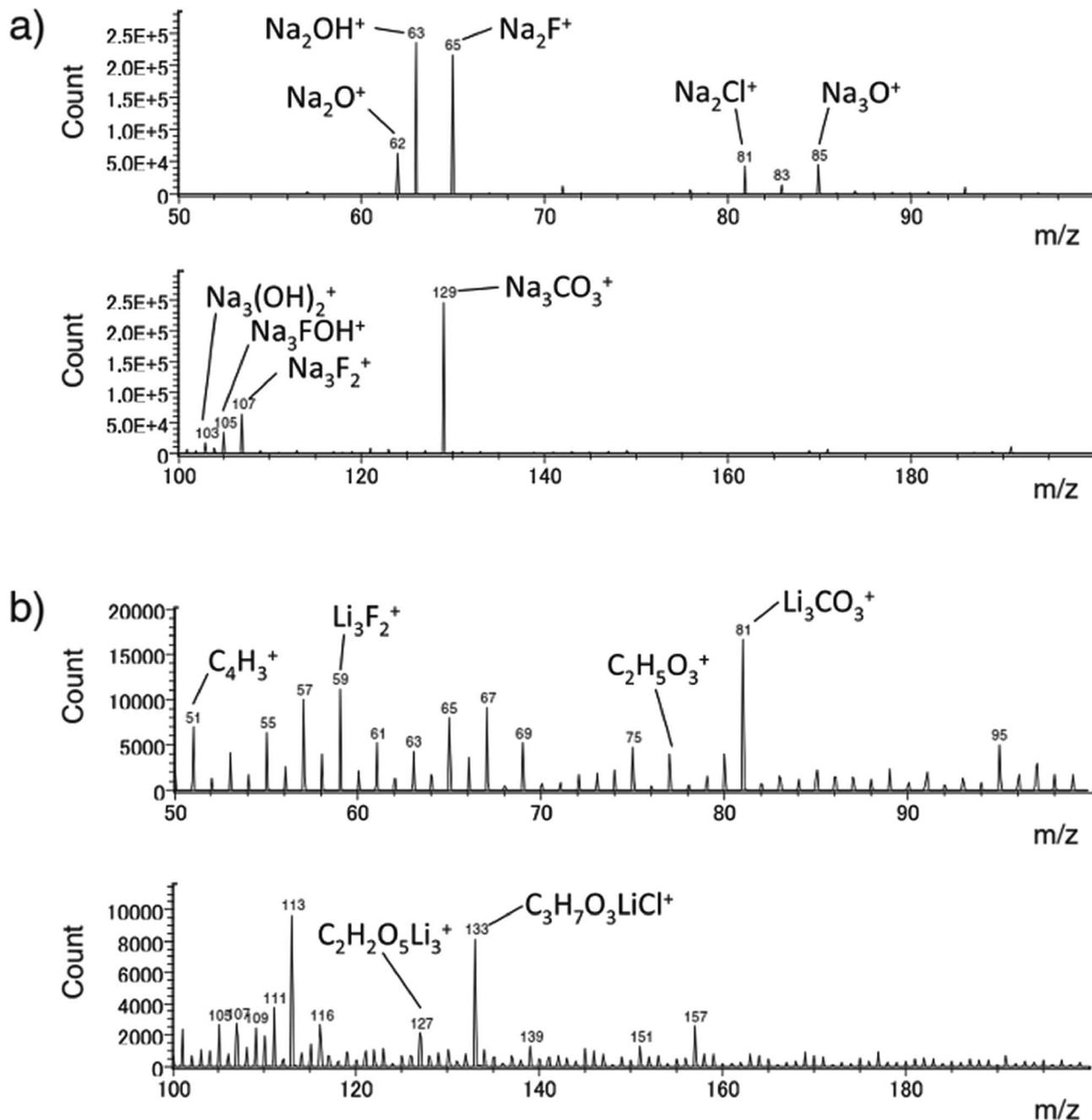
Fig. 21 TOF-SIMS positive ion spectra for the hard-carbon electrodes after the first galvanostatic cycle in (a) sodium and (b) lithium cells. Reproduced with permission<sup>128</sup> © 2011, WILEY-VCH Verlag GmbH & Co.
