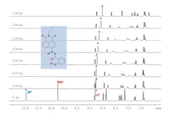
Fig. 7  $^{1}$ H NMR titration of probe 2 with TBAF in DMSO- $d_{6}$ . [2] = 10.7 mM.
