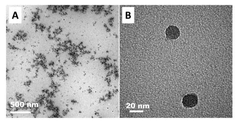
Fig. 6 TEM images of the colloidal dispersion of 1/C<sub>60</sub> obtained by HSVM.
