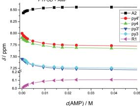
Fig. 6 <sup>1</sup>H NMR titration of PHENPOD (up) and PYPOD (down) with AMP, pD 6.8. For atom labelling see Scheme 1 and Fig. 5.
