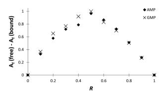
Fig. 3 Job plot for complex formation between PHENPOD and AMP (\*) or GMP (X). Spectra were recorded at 369 nm in a pH 5.0 solution (0.05 M cacodylate buffer) at a total concentration of [PHENPOD] + [NMP] =  $5 \times 10^{-5} M.$
