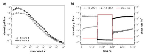
Fig. 3 (a) Steady shear rheological measurements reveal the response to increasing shear stress of solutions and hydrogels with 1.0 wt% and 1.5 wt% 1. (b) Step-rate measurements of samples with 1.0 wt% and 1.5 wt% 1 display the different recovery of the hydrogel network immediately after the breakdown due to a high magnitude shear rate.
