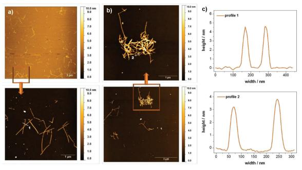
Fig. 5 AFM images of 100-fold diluted hydrogel with 1.5 wt% 1 at (a) pH 4 and (b) pH 6 show rod like structures which assemble in a different manner. (c) The height profiles 1 and 2 were marked within the zoom images. Silicon wafers were used as substrate.
