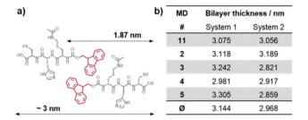
Fig. 7 (a) Schematic representation of the estimated membrane thickness from the calculated length of peptide 1 taking into account overlapping Fmoc-protection groups in the core of the bilayer. (b) Average thickness of the bilayer models of peptide 1 and 2, calculated from 100 evenly distributed snapshots for each independent 5 ns MD run.
