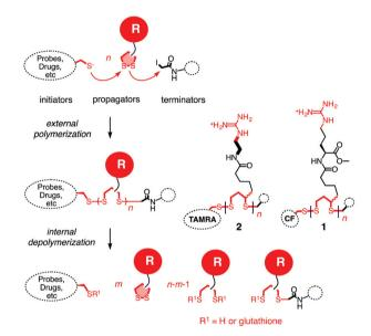
Fig. 1 The concept of substrate-initiated CPDs. Fluorescent initiators were used to initiate the polymerization through ring-opening disulfide exchange between guanidinium-containing propagators. The polymerization was guenched using jodoacetamide as the terminator.
