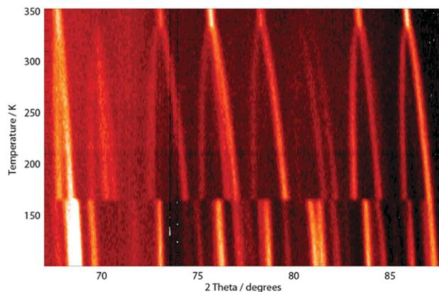
**Fig. 3** Stacked plot, viewed vertically, of part of the NPD data (67–88°) collected from MAPbI<sub>3</sub> over the temperature range 100–352 K. Peaks are shown as white and pale orange on a black background. The phase changes at 165 and 327 K are clearly observed as is the overall unit cell expansion.
