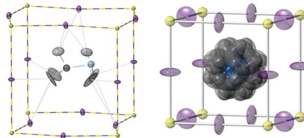
**Fig. 2** Left: one orientation of the MA<sup>+</sup> cation in the tetragonal phase of MAPbI<sub>3</sub> at 180 K; the cation is four-fold orientationally disordered around the *c*-axis which is vertical in this diagram. Right: orientational disorder modelled in the cubic phase at 352 K. Atom key as in Fig. 1 and ADP ellipsoids at 50% probability.
