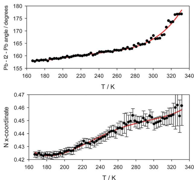
Fig. 5 Top – variation in the Pb–I<sub>2</sub>–Pb angle as a function of temperature in the tetragonal phase. Bottom – methylammonium nitrogen atom  $x$ -coordinate over the same temperature range.
