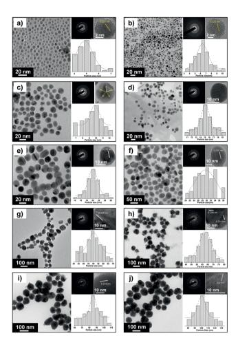
Fig. 3 FEG-TEM images of silver nanoparticles of various size ranges (a)  $5\pm0.7$  nm; (b)  $7\pm1.3$  nm; (c)  $10\pm2.0$  nm; (d)  $15\pm2.3$  nm; (e)  $20\pm2.5$  nm; (f)  $30\pm5.1$  nm (g)  $50\pm7.1$  (h)  $63\pm7.6$  (i)  $85\pm8.2$  (j)  $100\pm11.2$ . For each image, the corresponding high resolution (HRTEM) image and lattice fringes (*d*-spacing) are shown. The histograms show the range of particle size distribution.
