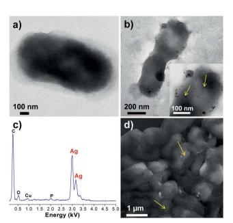
Fig. 7 FEG-TEM images of *E. coli* cells (a) untreated and (b) after treatment with silver nanoparticles. Inset shows the magnified image with the presence of silver nanoparticles, as shown by arrows. EDX analysis (c) of the bacteria shows the presence of silver. The FEG-SEM image (d) further confirms the presence of silver all over the bacterial surface.
