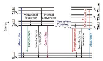
Fig. 2 Jablonski energy level diagram showing principal luminescence processes in an organic molecule (left: singlet manifold; right: triplet manifold). The full and dotted arrows represent radiative and non-radiative processes.
