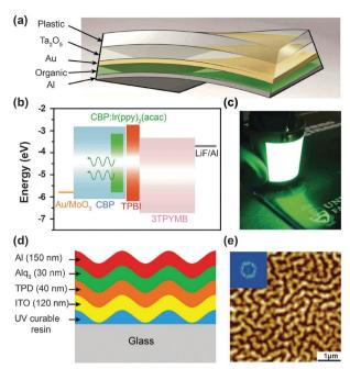
Fig. 19 (a) Device configuration of a PHOLED using  $Ta_2O_5$  as the light out-coupling layer. (b) The energy level diagram of active layers used in PHOLEDs. (c) The photographic image of the device in operation. (d) A quasi-periodic buckling structure designed for enhancing light out-coupling. (e) Topographic AFM image of buckling patterns formed by a 10 nm-thick aluminium layer. (Reproduced with permission from ref. 117a and b. Copyright 2011 and 2010, Nature Publishing Group.)
