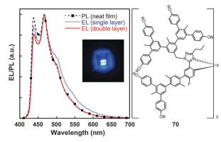
Fig. 6 Photoluminescence (PL) and electroluminescence (EL) spectra of 70 (inset: the corresponding digital image of the device derived from 70). (Reproduced with permission from ref. 38. Copyright 2009, American Chemical Society.)
