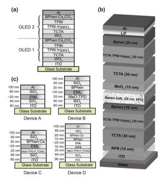
Fig. 17 Device configurations of tandem OLEDs using organic-inorganic hybrids, including (a) BPhen:Cs<sub>2</sub>CO<sub>3</sub>, (b) BPhen:CsN<sub>3</sub> and (c) BPhen:Cs, as the charge generation layer. (Reproduced with permission from ref. 109-111. Copyright 2010 and 2012, Wiley-VCH Verlag GmbH & Co. KGaA.)
