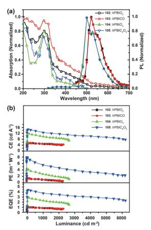
Fig. 10 (a) Absorption and photoluminescence spectra of 102-105 dissolved in dilute  $CH_2Cl_2$  solution. (b) The corresponding efficiency curves of the PHOLEDs derived from 102-105. (Reproduced with permission from ref. 53. Copyright 2011, Royal Society of Chemistry.)
