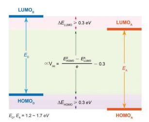
**Fig. 23** Schematic drawing of the donor and acceptor energy levels for the OPV devices.
