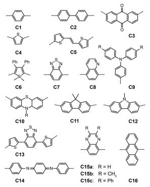
Fig. 25 Conventional building blocks for OPVs.
