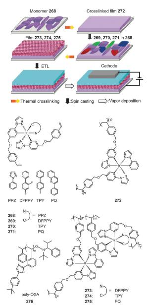
Fig. 18 procedure of solution-processed multi-layer devices on the basis of crosslinkable monomers 268-271 and the corresponding crosslinked polymers **272–275**. (Reproduced with permission from ref. 116. Copyright 2009, Wiley-VCH Verlag GmbH & Co. KGaA.)
