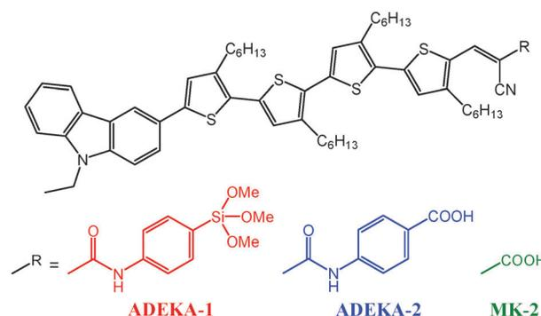
**Fig. 1** Molecular structures of carbazole dyes with a trimethoxysilyl group (**ADEKA-1**) and with a carboxy group (**ADEKA-2** and **MK-2**) as the anchor moiety for chemical bonding to the surface of the TiO<sub>2</sub> electrodes.
