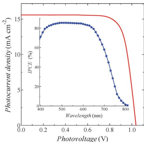
Fig. 3 Typical  $I$ - $V$  properties of the **ADEKA-1**-sensitized solar cell with the highest efficiency of 12.5% (entry 8 in Table 1) under the simulated one sun irradiation (AM-1.5G,  $100 \text{ mW cm}^{-2}$ ). Inset shows the IPCE spectrum of the cell.
