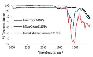
Fig. 1 FR-IR spectra of Fe $_2$ O $_3$  1, SiO $_2$ -coated Fe $_2$ O $_3$  2, and iodoalkyl-functionalized SiO $_2$ -coated MNPs 3.
