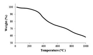
Fig. 4 TGA curve of MNPs 7.
