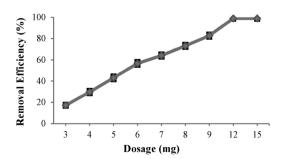
Fig. 6 Effect of MNPs 7 dosage on extraction of Cu(II).
