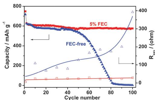
**Fig. 3** Changes of the cycling capacities and SEI film resistances of the Sb/C anodes in the 1.0 mol L<sup>-1</sup> NaPF<sub>6</sub> + EC-DEC electrolyte with (red ■ □) and without (blue ▲ △) the addition of 5% FEC additive.
