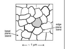
would be expected if *all* the electrode surface was uniformly active in the electrolysis. Rather the unusual and characteristic voltammograms were consistent with a model in which the electrode surface acted, in effect, as an "array of microband electrodes" in
