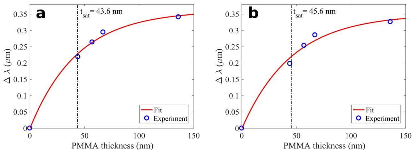
**Fig. 4** Measurements of the penetration depth  $t_{\text{sat}}$  of the metasurface evanescent field using variable-thickness PMMA coverage. The wavelength shift  $\Delta\lambda$  of the reflectivity maximum for (a) Pixel 1, and (b) Pixel 2 depends on the PMMA thicknesses  $t$ . At  $t = t_{\text{sat}}$  the shift reaches 63% of its asymptotic value.
