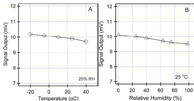
**Figure 8** Effect of the temperature (A) and relative humidity (B) on the signal output of the sensor (methane concentration: 50%LEL)
