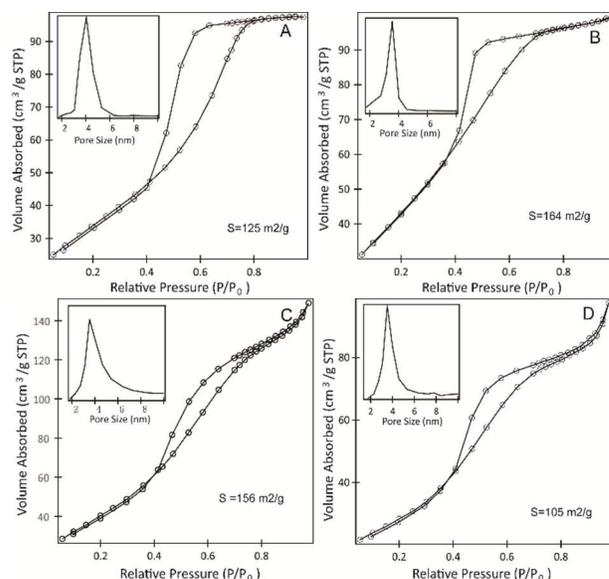
Figure 4 N<sub>2</sub> adsorption-desorption isotherms and corresponding pore size distributions of mesoporous PdO/Pt/Al<sub>2</sub>O<sub>3</sub> hybrid with different mole ratio of noble-metal/Al: (a) 1/4, (b) 1/2, (c) 1/1, (d) 2/1
