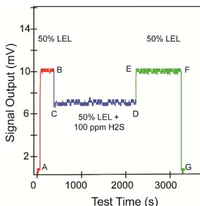
**Figure 9** Response of the sensor (methane concentration: 50%LEL) before (A-B) and after (E-F) the exposure to 100 ppm H<sub>2</sub>S, and the response under the exposure to 100ppm H<sub>2</sub>S mixed with 50%LEL methane (C-D).
