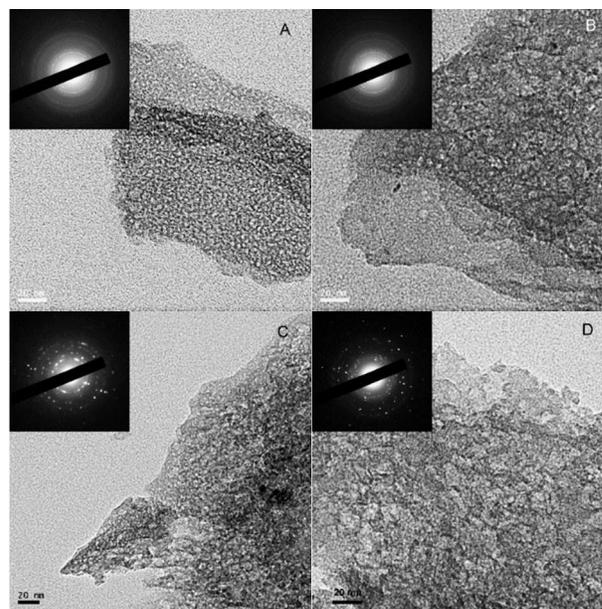
Figure 1 TEM images of mesoporous PdO/Pt/Al<sub>2</sub>O<sub>3</sub> hybrids with different mole ratio of noble-metal/Al (a) 1/4, (b) 1/2, (c) 1/1, (d) 2/1
