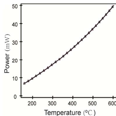
**Figure 7** Power consumption of the micro-heater as a function of working temperature of the gas sensor
