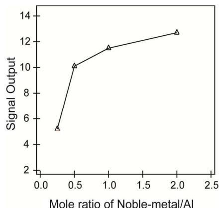
**Figure 5** Responses of the MEMS sensor based on PdO/Pt/Al<sub>2</sub>O<sub>3</sub> hybrids with different mole ratio. (25 °C, 25% RH, 2 vol% methane or 50% of the lower explosion limit, 50% LEL)
