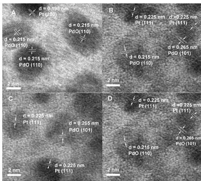
Figure 2 HRTEM images of mesoporous PdO/Pt/Al<sub>2</sub>O<sub>3</sub> hybrid with different mole ratio of noble-metal/Al (a) 1/4, (b) 1/2, (c) 1/1, (d) 2/1
