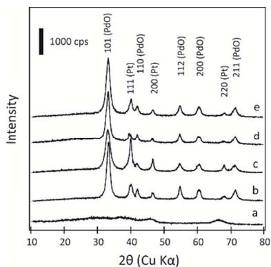
Figure 3 Wide angle XRD pattern of mesoporous PdO/Pt/Al<sub>2</sub>O<sub>3</sub> hybrid with different mole ratio of noble-metal/Al (a) 0/1, (b) 1/4, (c) 1/2, (d) 1/1, (e) 2/1
