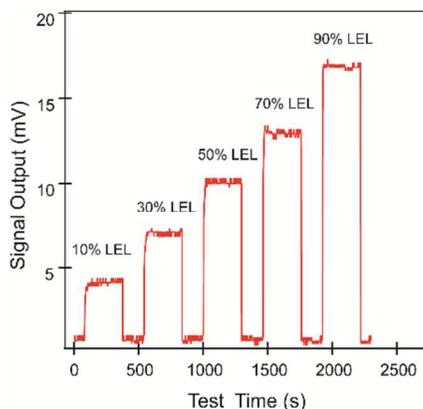
**Figure 6** Sensor responses to the methane inputs of different concentrations (25 °C, 25% RH)
