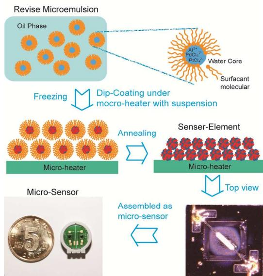
Scheme 1. Reverse micro-emulsion and pyrolysis protocol for fabricating PdO/Pt/Al<sub>2</sub>O<sub>3</sub> porous film on MEMS micro-heater chip
