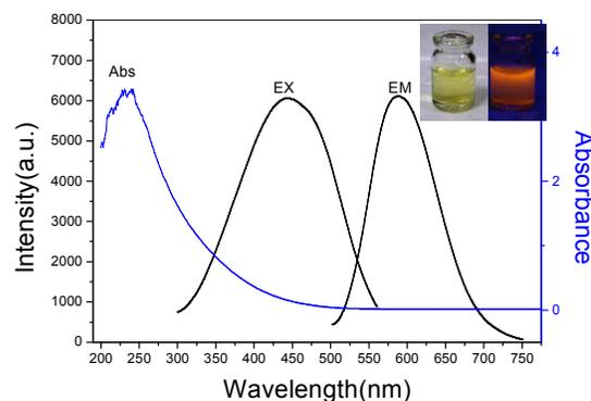
NCs. Inset: Photographs of an aqueous solution of AuAg NCs under visible light (left) and UV irradiation (λ = 365 nm) (right).
