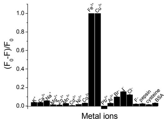
**Fig 3.** The fluorescence intensity ratio of changes of the AuAg NCs induced by various ions and biological molecules ( $1 \times 10^{-4} \text{M}$ ),  $F_0$  is the initial intensity of AuAg NCs and  $F$  is the fluorescence after the addition of metal ions, the error bars represent the standard deviation of three measurements.
