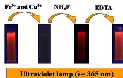
**Scheme 1.** Schematic diagram of successive detection of  $\text{Fe}^{3+}$  and  $\text{Cu}^{2+}$  based on the binary fluorescence sensor of AuAg NCs.
