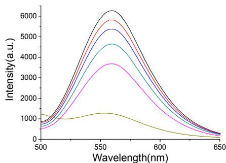
**Fig 4.** Fluorescence quenching of AuAg NCs with increasing  $\text{Fe(III)}$  concentration (from top to bottom:  $0 \text{M}$ ,  $2 \times 10^{-8} \text{M}$ ,  $1.9 \times 10^{-7} \text{M}$ ,  $7.2 \times 10^{-6} \text{M}$ ,  $3.5 \times 10^{-5} \text{M}$ ,  $1.7 \times 10^{-4} \text{M}$ ).
