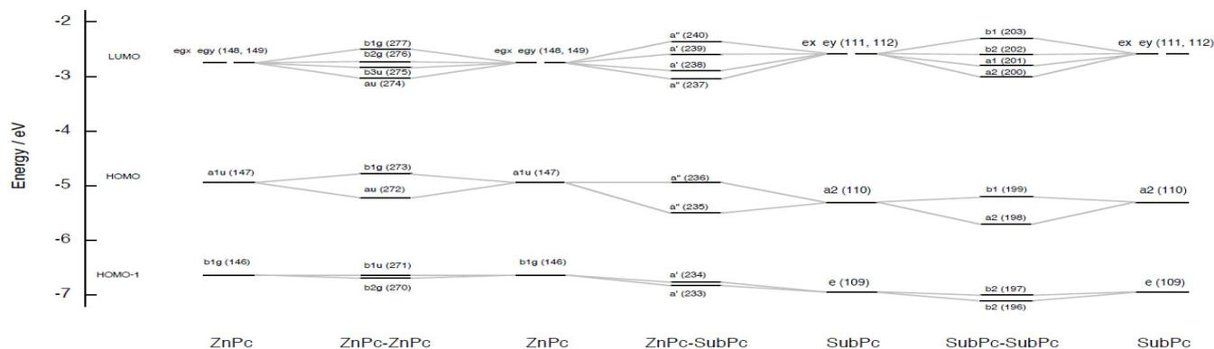
**Fig. 4** Partial molecular orbital energy diagram for ZnPc-ZnPc, ZnPc-SubPc, and SubPc-SubPc, and for ZnPc and SubPc, and their mutual relationship. The numbers in the parentheses indicate orbital number.
