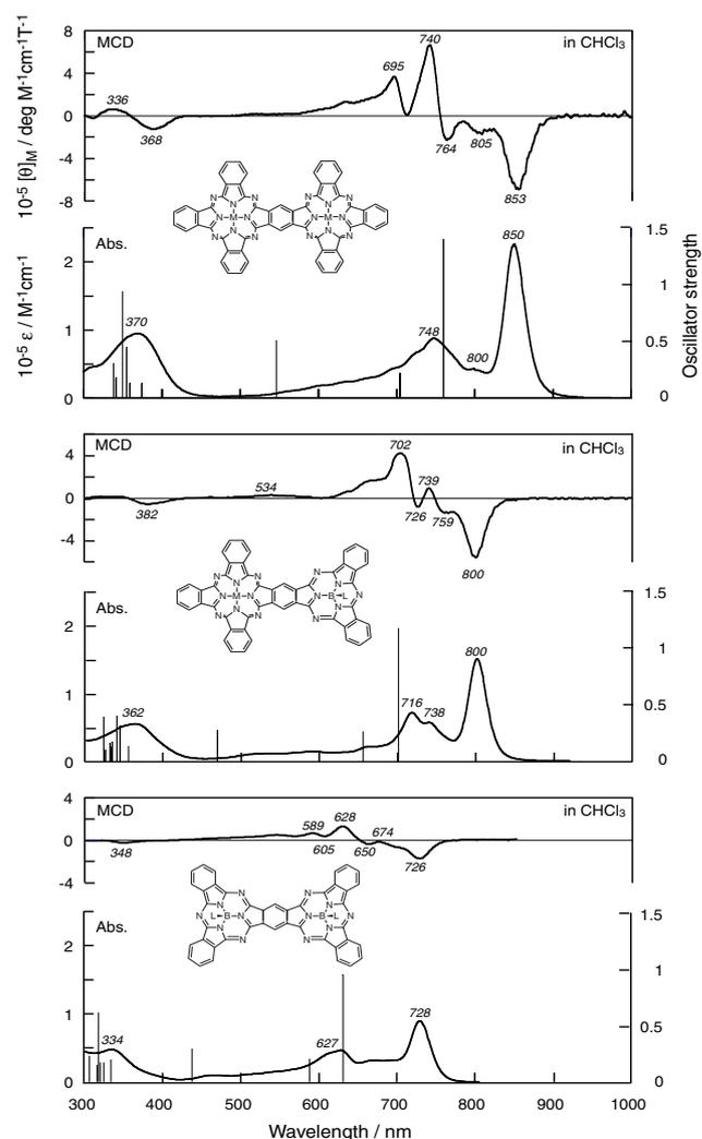
Fig. 3 Electronic absorption and magnetic circular dichroism (MCD) spectra of ZnPc-ZnPc **2** (top), ZnPc-SubPc **1** (middle), and SubPc-SubPc **3** (bottom) in  $\text{CHCl}_3$ . All compounds contain  $\text{OCH}_2\text{CF}_3$  groups as substituents, but these are omitted in the structure.
