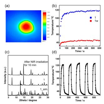
Fig. 7 (a) IR camera images of 1 during NIR light exposure (850 nm, 0.3 W cm<sup>-2</sup>). (b) Photothermal conversion curves for 10 min. (c) PXRD patterns before and after NIR irradiation. (d) Cyclic photothermal curve upon NIR exposure.
