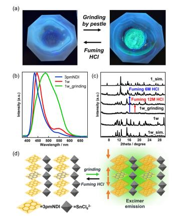
Fig. 6 (a) Mechanochromism observed in 1w. (b) Emission spectra of 3pmNDI and 1w before and after grinding, with  $\lambda_{ex}$ = 350 nm. (c) PXRD patterns of 1w, showing changes before and after grinding, and exposure to HCl vapor. (d) A schematic illustration depicting mechanochromism caused by excimer emission.
