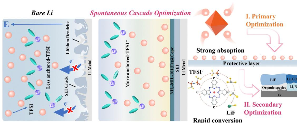
Fig. 1 Schematic diagram of the principle of the modification layer NH<sub>2</sub>-MIL-101(Fe)@Copc.
