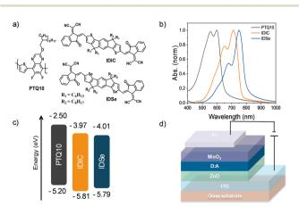
Fig. 2 (a) Chemical structures of PTQ10, IDIC and IDSe; (b) normalized absorbance of the neat materials; (c) energy levels of the materials extracted from PESA measurements; (d) schematic of the BHJ donoracceptor device structure with inverted architecture
