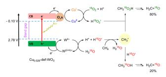
Fig. 21 Proposed mechanism for charge transfer steps during selective  $CH_4$  oxidation over  $Cu_{0.029}$ -def-WO<sub>3</sub>.
