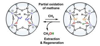
Fig. 20 Strategy used to generate monomeric [Cu]<sup>2+</sup> sites in a pure alumina environment and the subsequent reaction with CH<sub>4</sub> to form hydroxyl and methoxy species.
