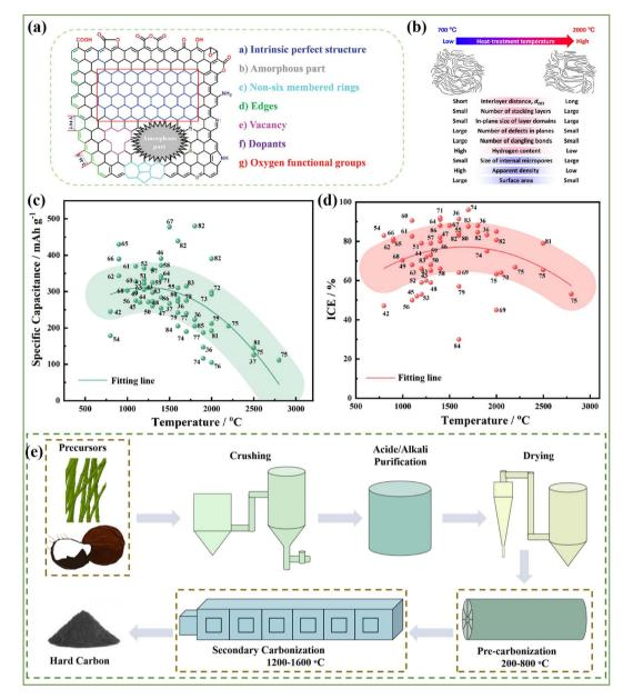
Fig. 5 (a) Illustration of carbon surface with different types of defects. (b) Diagram of structural parameters for HC synthesized at 700 °C and 2000 °C. (c and d) Relationship of specific capacity and ICE with the pyrolysis temperature of HCs based on published works. (e) Schematic illustration of the main steps for a mature route to HC commercialization.
