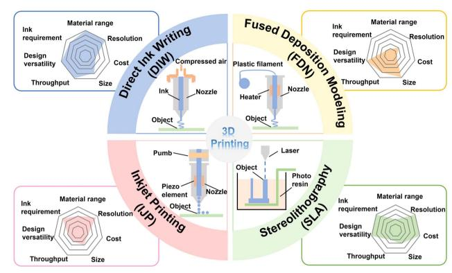
Schematic of printing and characteristics of four representative 3D printing techniques (DIW, FDM, IJP and SLA) to fabricate MBs
