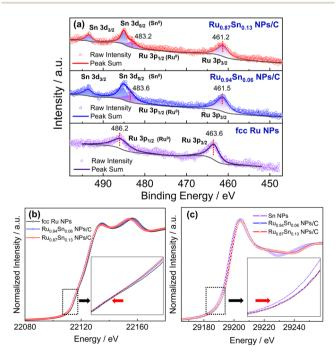
Fig. 5 (a) Ru 3p XPS spectra of fcc Ru NPs, Ru<sub>0.94</sub>Sn<sub>0.06</sub> NPs/C and Ru<sub>0.87</sub>Sn<sub>0.13</sub> NPs/C. The black curves serve as the background files. (b) Ru K-edge XANES spectra of fcc Ru NPs, Ru<sub>0.94</sub>Sn<sub>0.06</sub> NPs/C and Ru<sub>0.87</sub>Sn<sub>0.13</sub> NPs/C. (c) Sn K-edge XANES spectra of Sn NPs,  $\mbox{Ru}_{0.94}\mbox{Sn}_{0.06}$  NPs/C and  $\mbox{Ru}_{0.87}\mbox{Sn}_{0.13}$  NPs/C.
