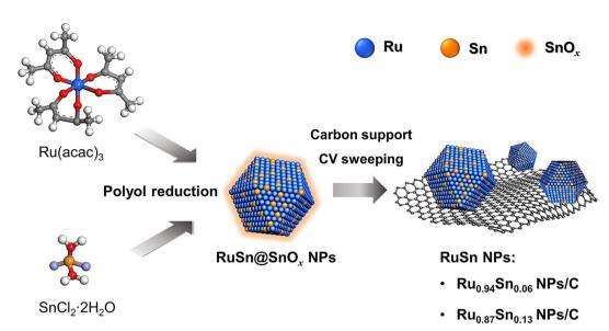
Scheme 1 Synthesis of RuSn solid-solution alloy NPs from cyclic voltammetry sweeping of RuSn@SnO<sub>x</sub> NPs.
