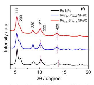
Fig. 2 Atomic-resolution HAADF-STEM images of (a)  $Ru_{0.94}Sn_{0.06}$  NPs/C and (b)  $Ru_{0.87}Sn_{0.13}$  NPs/C. (c) FFT pattern of (a). (d) Expanded image of the red dashed square region in (a). (e) Expanded image of the red dashed square region in (b). (f) Synchrotron XRD patterns of Ru NPs,  $Ru_{0.94}Sn_{0.06}$  NPs/C and  $Ru_{0.87}Sn_{0.13}$  NPs/C. The radiation wavelength is 0.2069(1) Å.
