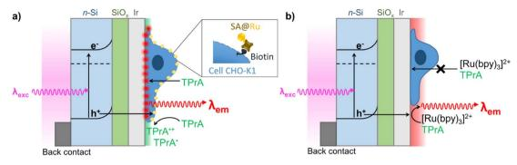
Fig. 1 Schematic representation of two PECL microscopy modes for imaging single cells with back-illumination configuration. (a) Direct imaging by PECL+ of cell membrane labeled with the streptavidin-modified [Ru(bpy)<sub>3</sub>]<sup>2+</sup> luminophore (SA@Ru) in TPrA solution; and (b) label-free imaging of cells by PECL— with cells immersed in a PBS solution containing both [Ru(bpy)<sub>3</sub>]<sup>2+</sup> and TPrA.
