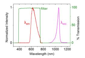
Fig. 3 Spectra of the 1050 nm LED excitation (purple curve), the resulting PECL emission (red curve), and the filter transmission (green curve).
