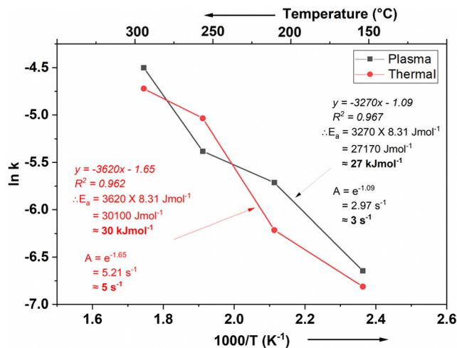
Fig. 9 Arrhenius plot for  $\text{NH}_3$  reaction on a TDMAA-terminated surface, emitting dimethylamine, in plasma (black line) and thermal (red line) processes, during the  $\text{NH}_3$  pulse. Straight lines (not shown) represent a weighted linear fit to the data, from which the corresponding Arrhenius parameters were drawn.
