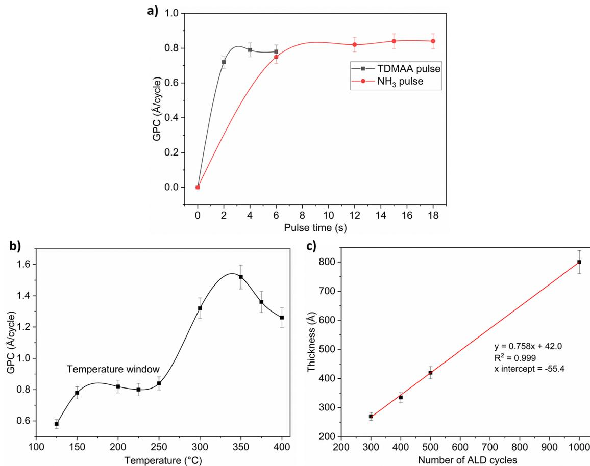
Fig. 2 Saturation curves for the thermal process, showing the effect of the TDMAA pulse time and the NH<sub>3</sub> pulse time on the GPC (a). The thermal process growth dependence on process temperature is shown in (b) while film thickness dependence on number of cycles, showing no nucleation delay, for the thermal process is illustrated in (c).
