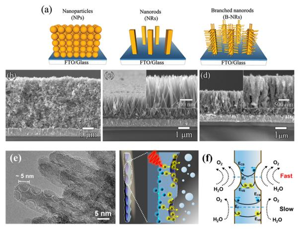
Fig. 5 (a) Schematic diagram of the synthesis of  $TiO_2$  branched nanorods. SEM images of (b)  $TiO_2$  nanoparticles, (c) nanorods, and (d) branched nanorods. Reprinted with permission from ref. 43. Copyright © 2011, American Chemical Society. (e) TEM image of the TiO<sub>2</sub> nanowire arrays. (f) Schematic illustrations of the hole extraction effect of TiO<sub>2</sub> nanowire arrays. Reprinted with permission from ref. 45. Copyright © 2022, American Chemical Society.
