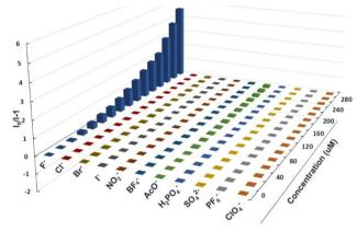
Fig. 4  $(I_0/I)$ -1 of 11 anions for the emission of **3a** in THF (10  $\mu$ M in THF) at different equivalents of anions.
