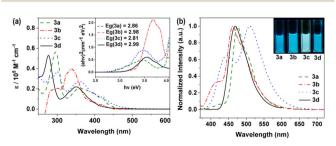
Fig. 1 UV-Vis absorption spectra (left) and photoluminescence (PL) spectra (right) of the phenothiazine derivatives in THF solutions; the extrapolated optical band gaps ( $E_g$ ) is shown as insets.
