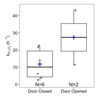
Fig. 4 Statistics of  $k_{\rm H_2O_2}$  for regular cleaning of the near counter under different ventilation conditions. The box and whisker plots show the median (line), mean (blue marker), first and third quartiles (box), and minima and maxima (whiskers). The number under each box and whisker plot indicates the number of cleaning events for that condition.
