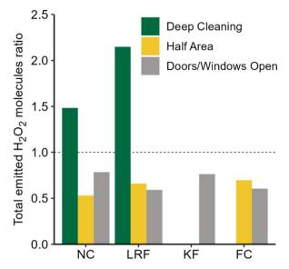
Fig. 5 Ratio of total emitted  $H_2O_2$  molecules under the cleaning conditions investigated (deep cleaning, half area, and door/windows open) to the standard controlled cleaning condition.
