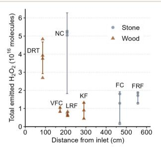
Fig. 2 Total emitted  $H_2O_2$  as a function of average distance from inlet for controlled regular cleaning events. Abbreviated texts indicate surface types listed in Table 1. Error bars represent the standard deviation about the mean.
