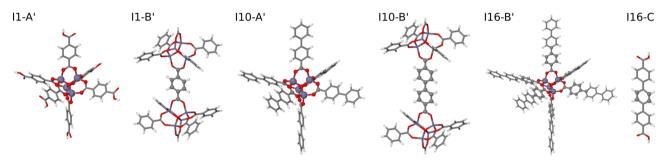
Fig. 5 Extended large molecular fragments of IRMOF-1, -10, and -16 with an increased number of atoms in bulk-like environments. The molecular fragment structures are represented by sticks, while the central atoms of the fragments embedded in a bulk-like environment up to a radius of  $R_{\rm frag}^{\rm conv}$ 8.718 Å are shown as balls. The fragments I1-B' and I16-C' are identical to their counterparts shown in Fig. 4.
