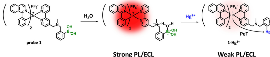
Scheme 1 The detection mechanism of probe 1 for \text{Hg}^{2+} ions.
