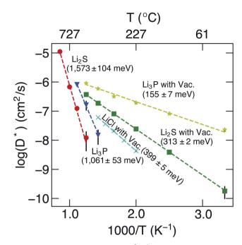
Fig. 3 Arrhenius plots of  ${\rm Li}^+ D^*$  (in cm² s $^{-1}$ ) of bulk binary compounds from MTP-MD simulations. The activation energies, calculated from eqn (7), and the related error bars are provided as text annotations. Vac. stands for structures with a Li vacancy.
