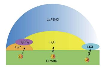
Fig. 5 Schematic illustration of a possible structure of the interface between Li metal and argyrodite-Li<sub>6</sub>PS<sub>5</sub>Cl, as inferred from the interfacial energetics and Li-ion transport simulations.
