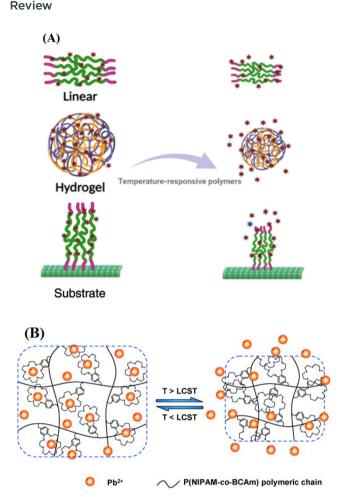
**Fig. 5** (A) Schematic illustration for temperature-responsive polymers exceeding their LCST and (B) temperature-responsivity of the P(NIPAM-co-BCAm) hydrogel above the LCST which allows the hydrogel to release the adsorbed ions. <sup>55</sup> Copyright 2009, Reproduced with permission from Elsevier Ltd.
