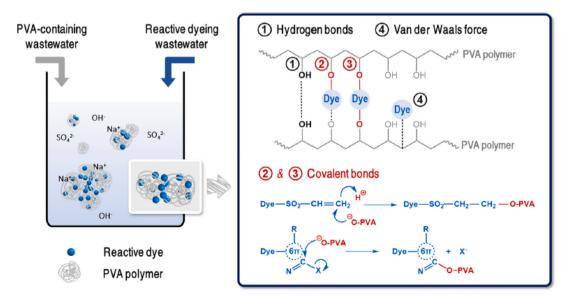
Fig. 8 Adsorption mechanism of the crosslinking-induced precipitation of PVA from wastewater through the hydrogen bonding and van der Waals interactions, <sup>61</sup> Copyright 2014, Reproduced with permission from the Royal Society of Chemistry (RSC).
