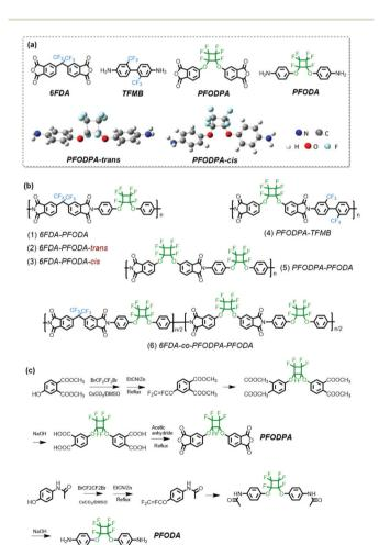
**Scheme 1** (a) Chemical structures of polyimide monomers studied in this work and the optimized conformations of the PFODA isomers. (b) Chemical structures of the synthesized polyimides. (c) Synthesis routes for the PFCB-containing monomers.
