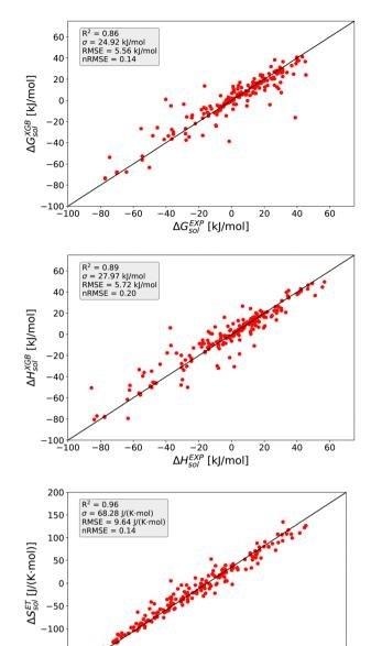
Fig. 2 Goodness of fit plots for predicted and experimental values (subscript EXP): XGB model for  $\Delta G_{\rm sol}$  (top), XGB model for  $\Delta H_{\rm sol}$  (middle) and ET model for  $\Delta S_{sol}$  (bottom). The straight black lines highlight a full coincidence.
