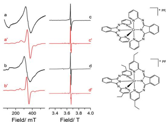
**Fig. 2** Experimental and simulated EPR spectra of (a and c)  $[\text{Cr}(\text{bpi-1})_2]\text{PF}_6$  and (b and d)  $[\text{Cr}(\text{bpi-2})_2]\text{PF}_6$  recorded as 1% doped solids in their corresponding diamagnetic cobalt matrix. Experimental data were recorded at (a and b) X-band frequency, 140 K, and (c and d) W-band frequency, 20 K.
