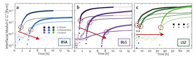
Fig. 1 Interfacial shear time sweeps of the network formation of (a) BSA, (b) BLG, and (c) LSZ at the n-octane, 1-chlorooctane, and 1-octanol interfaces. Red circles indicate the cross-over time and the red arrows indicate the increase in oil polarity. Data for BLG are taken from an earlier publication.<sup>29</sup> The equilibrated moduli of BLG and BSA at n-octane after 10 h are extrapolated with dotted lines
