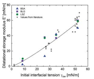
Fig. 2 Elastic dilatational modulus E' of BSA, BLG, and LSZ plotted over  $\gamma_{\rm ow}$ . The black dotted line represents the fit for all globular proteins (eqn (1)) including values from the literature, <sup>27,29,56–62</sup> listed in the ESI† (Table S1).
