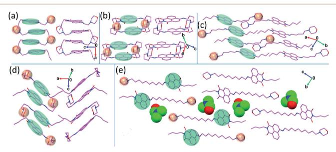
Fig. 1 Representation of the solid-state geometry of the synthesized NIMCs, (a) NIMC2, (b) NIMC3, (c) NIMC5, (d) NIMC4 and (e) NIMC10 obtained from the single-crystal X-ray diffraction. Crystal packing reveals that the molecules are stacked  $via \pi \cdots \pi$  interactions and the shorter alkyl spacers adopt a bent chain conformation, while a straight chain geometry is adopted by intermediate and longer alkyl spacers.
