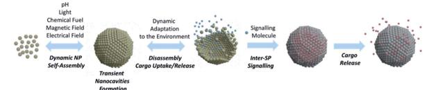
Fig. 10 Schematic representation of NP dynamic self-assembly leading to the formation of SP endowed with inner nanocavities. The obtained SP can further adapt dynamically to the surrounding environment affording a conformational rearrangement with possible cargo release/uptake. Furthermore, released cargos can potentially act as signalling molecules for another SP, triggering the release of a second cargo.
