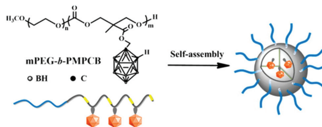
Scheme 1 Structure of the amphiphilic carborane-conjugated polycarbonate and self-assembly in water, adapted from ref. 20 with permission from the American Chemical Society, copyright 2016.
