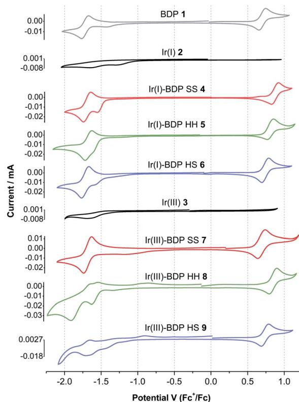
Fig. 7 Cyclic voltammograms of the parent compounds BDP 1, Ir(i) 2 and Ir(III) 3, and the bifunctional catalysts 4–9, measured in a 0.1 M solution of TBA- $BAR_4^F$  in dichloromethane under argon. Ferrocene was used as internal standard. Scan rate: 100  $mV s^{-1}$ .
