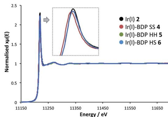
Fig. 8 The XAS spectra at the Ir L<sub>3</sub> edge for the Ir(I) based complexes.
