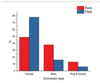
Fig. 9 (red) Proportion of packs utilising each intermodular connection type, (blue) proportion of connection type across fleet population of modules. Data from 2018 EU sales of (H)EVs where available.
