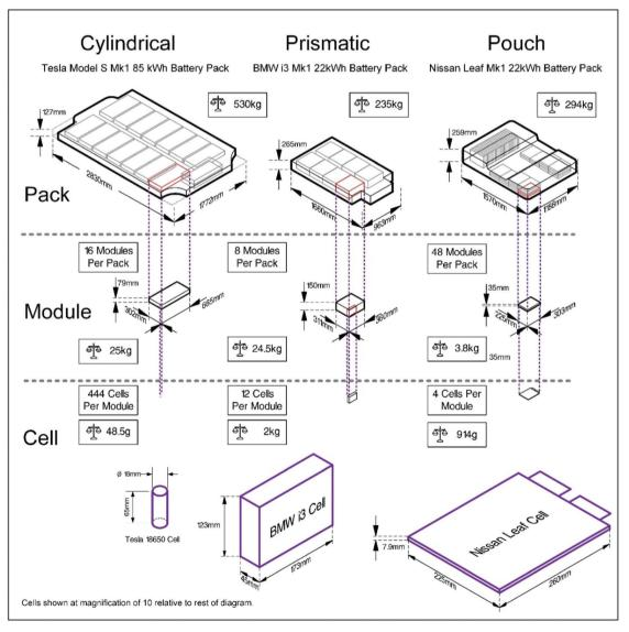
Fig. 3 Different types of battery cells and how they are organised to form modules and packs.<sup>32</sup>
