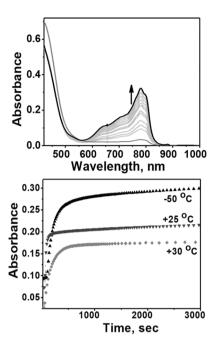
Fig. 4 Top: Spectral changes associated with the catalytic reduction of dioxygen by Co<sub>4</sub>L1 (0.04 mM) in the presence of Fc\* and TFA. Bottom: Time profiles of the formation of Fc\*+ monitored at 780 nm during the reduction of O2 (0.18 mM) by Fc\* (3 mM) and Co4L1 (0.04 mM) in the presence of TFA (10 mM) in acetone at 30 °C, 25 °C as well as at -50 °C.
