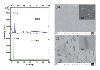
Fig. 4 (a) X-ray diffractograms of thin films of NIB and NIBD. FE-SEM images of NIBD (b) and NIB (c) formed by the evaporation of the respective aggregates from a 99.9% water–0.1% DMF mixture on aluminium foil at room temperature (10  $\mu\text{M}$ ).
