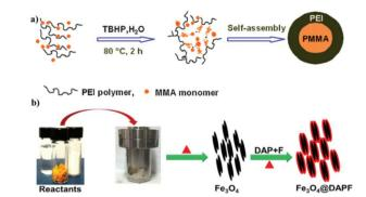
Fig. 1 (a) Synthesis of PMMA/PEI core—shell nanoparticles. Reproduced with permission from ref. 37. Copyright 2011 Elsevier. (b) Schematic Illustration of the Synthesis of  $Fe_3O_4$ @DAPF ferromagnetic nanorods. Reproduced with permission from ref. 38. Copyright 2015 American Chemical Society.
