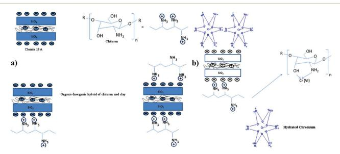
Fig. 8 (a) Organic-inorganic hybrid of chitosan and clay; (b) possible interaction mechanism of Cr(vi) with chitosan and organoclay. Reproduced with permission from ref. 108. Copyright 2011 Elsevier.
