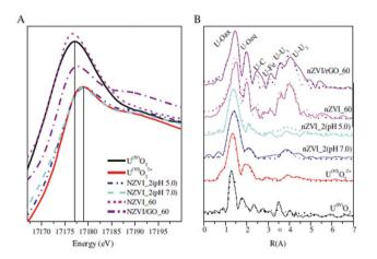
Fig. 9 XANES spectra (A) and Fourier transform (FT) of EXAFS spectra (B, solid and dashed lines: experimental and fitted data) for reference samples and U(vı)-reacted nZVI and nZVI/rGO composites,  $T=25\pm1\,^{\circ}\text{C}$ ,  $I=0.01\,\text{mol}\,\,\text{L}^{-1}\,\,\text{NaClO}_4\,\,\text{pH}=5.0$ . Reproduced with permission from ref. 174. Copyright 2014 Elsevier.
