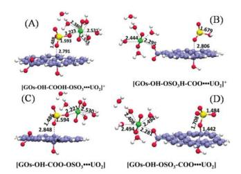
Fig. 10 Optimized models of GO complexes with uranyl species at pH = 2.0 (A and B) and at pH = 6.0 (C and D); bond lengths are in Å. Reproduced with permission from ref. 178. Copyright 2017 Elsevier.
