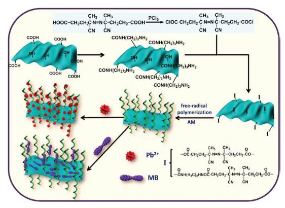
Fig. 5 Synthesis of PAM chains on RGO sheets, and Pb(II) and MB adsorption. Reproduced with permission from ref. 84. Copyright 2013 American Chemical Society
