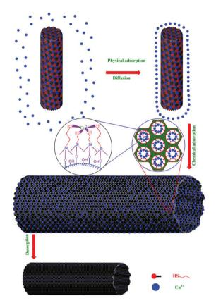
Fig. 6 The mechanism of Cu(ii) adsorption on PVA/SiO<sub>2</sub> nanofibers. Reproduced with permission from ref. 92. Copyright 2010 Elsevier.
