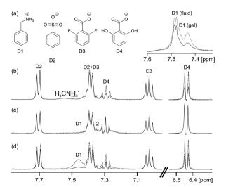
Fig. 4 (a) Structures of model drug compounds. (b–d) NMR spectra of model drug compounds in hydrogels recorded with (solid) and without (dashed) on resonance presaturation applied to the gel fibres: (b) 1/GdL hydrogel containing **D2–D4** and (inset top) hydrogel containing **D1** and NH<sub>4</sub>Cl. (c) 4 mg mL<sup>-1</sup> solution of **2** at pH 9 containing **D1–D4**. (d) Sample of (c) upon addition of 30 mM CaCl<sub>2</sub>.
