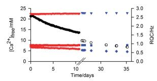
Fig. 6 Plots of  $[{\rm Ca}^{2+}]_{\rm free}$  in  ${\bf 2}/{\rm CaCl_2}$  gel versus time after an NaCl solution was placed on top of the sample. After the first solution (black circle) had stood on top of the gel for 26 days, the supernatant solution was removed, fresh solution placed on top and the second series of measurements (white) commenced. The RQCs of HDO (square), dioxane (down triangle) and formate (diamond) are plotted for the first (red) and second (blue) series of measurements.
