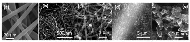
Fig. 1 SEM images of bare (a) and DWCNT (b), MWCNT (c), CVD-CNT (d) coated GDL, and n-GDL (e). (a) Reprinted from ref. 45 with permission from John Wiley & Sons, Inc. Copyright 2016 by John Wiley & Sons, Inc. (b) Adapted from ref. 40, Copyright 2009, The Electrochemical Society. (c) Reprinted from ref. 46 with permission from John Wiley & Sons, Inc. Copyright 2010 by John Wiley & Sons, Inc. (e) Reprinted from ref. 47, Copyright 2015, with permission from Elsevier.
