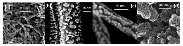
Fig. 4 SEM images of the Pt-CeO2 anode catalyst deposited on DWCNT (a), MWCNT (b), and CVD-CNT (c) coated GDL, and n-GDL (d). (a) Adapted with permission from ref. 40, Copyright 2009, The Electrochemical Society. (b) Reprinted with permission from ref. 51, Copyright 2012, Inderscience Enterprises Ltd. (d) Reprinted from ref. 47, Copyright 2015, with permission from Elsevier.
